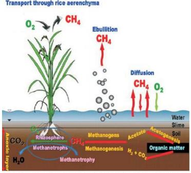
Figure 1: Schematic diagram of methane production, oxidation and
